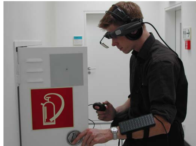
Mobile demonstrator: User testing the Xybernaut mobile assistant
